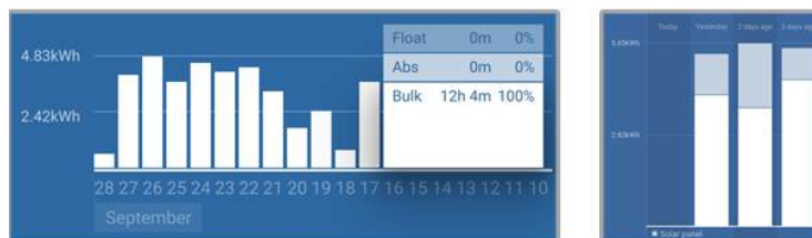
Left: Example of a system that is spending all its time in the bulk stage. Right: Breakdown of the charge stages - The system spends time in bulk and in the absorption stage.
