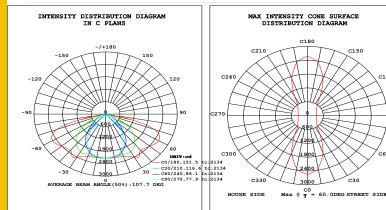
C Range: 0 - 90DEG C Interval: 5.0DEG Test Speed: HIGH Temperature:29.3DEG Operators: Test Date:2019-12-09
